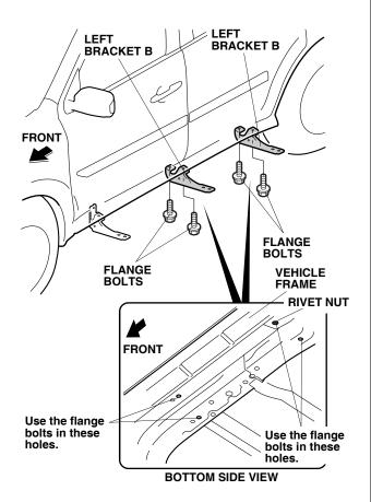
Position the left side step on the left bracket A and two left brackets B. Install the left side step with six flange bolts. Torque the flange bolts to 27 N·m (19 lbf·ft).
