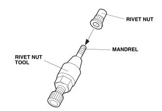
• Insert the rivet nut into the hole in the vehicle frame and install the hex wrench on the rivet nut tool.
